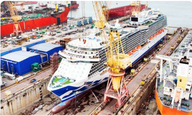
Royal Princess cruise ship undergoing drydocking works
