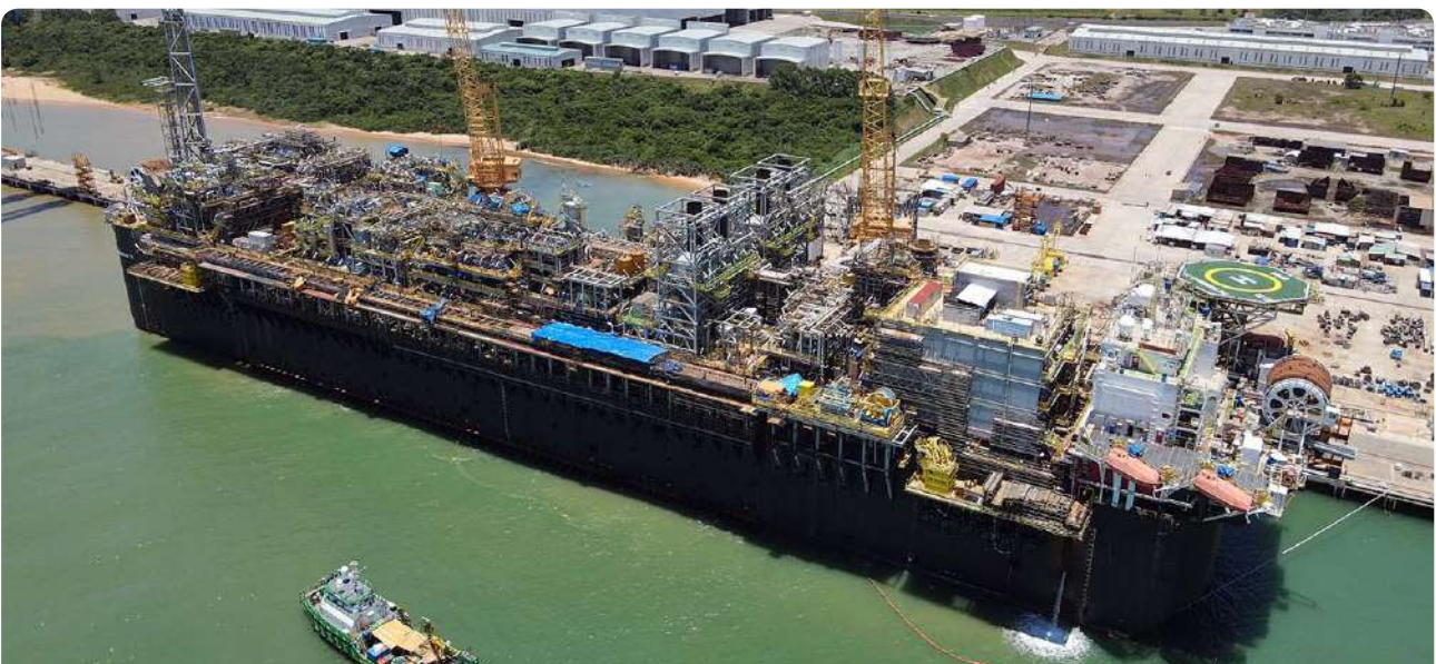
P-71 FPSO modification and topside modules work underway in our Brazil yard
