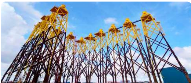
Completed fabrication of 11 wind turbine jacket foundations for the Formosa 2 Offshore Wind Farm in 2022, following the sailaway of four units in 2021
